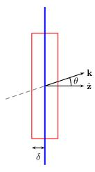
Figure 1: A plane wave with direction of propagation  $\mathbf{k}$  incident on a screen.
